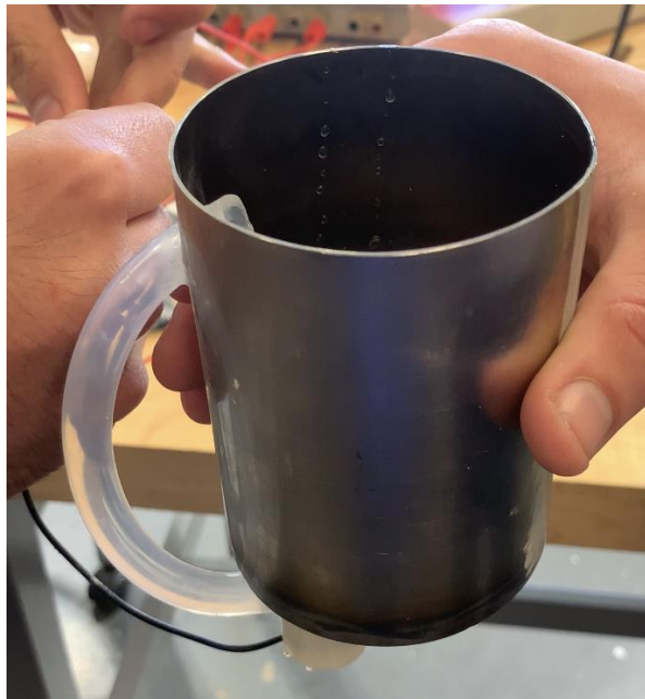
Figure 11: Inner Layer with Pump Attached
